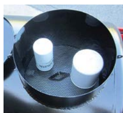
Rete scolafiltri interna. Filters drainage mesh.
